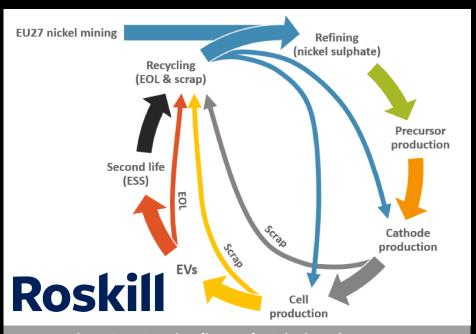
Desired EU27 circular flow of nickel in the domestic battery supply chain. Source: Roskill, 2020.
